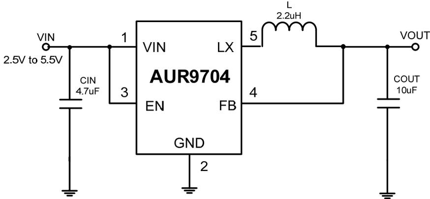
Figure1. Fixed Voltage Regulator
