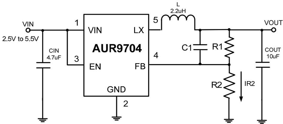
Figure2. Adjustable Voltage Regulator
