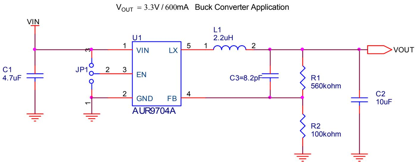
Figure4. The Evaluation Board Schematic
