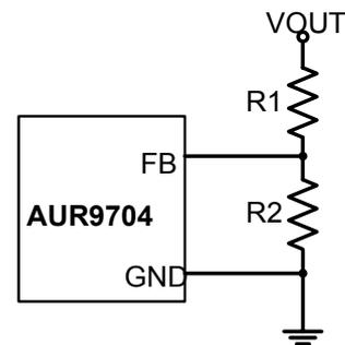
Figure3. Setting the Output Voltage
