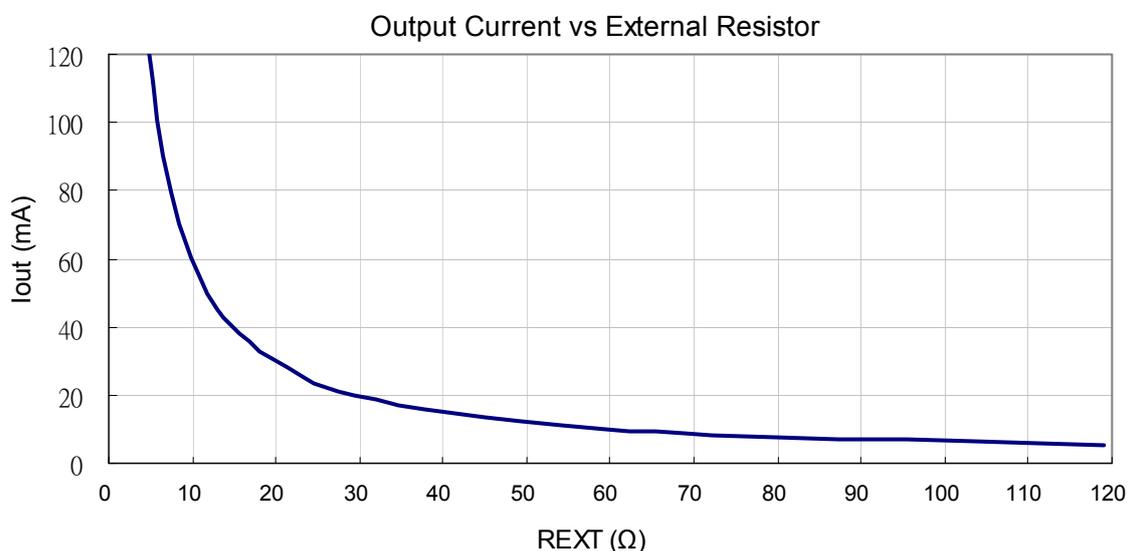
The output current is kept constant for driving multiple LEDs in series with each driver before reaching the dropout voltage limits. LEDs with various forward voltages ( $V_F$ ) can be used within usable voltage headroom. Typical output current characteristic of an output driver is shown below for illustrating driver dropout voltage vs. output current level.
